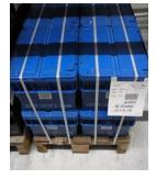
• Exception: for MU7 plastic straps must be routed in the middle row of handling unit in addition.
