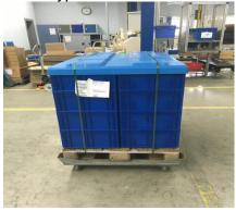
Non-self-adhesive label, fixed with max. 2 adhesive dots at MULTIPACK and 1 master label at front end fixed with max. 2 adhesive dots of defined types
